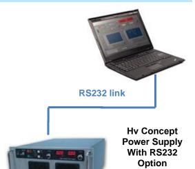
Control via COM-Port Any device with a RS232 com port can drive the generator.
